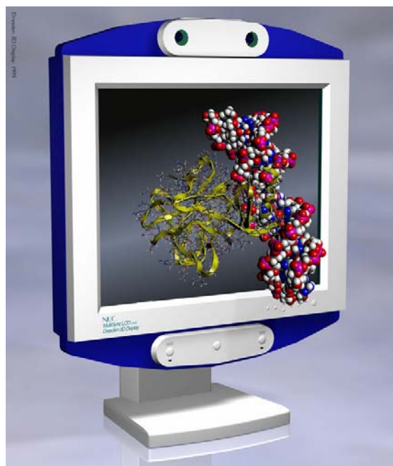
Pic 2: Autostereoscopic monitor. (Image downloaded from SeeReal Technologies GmbH (former Dresden3D) - http://www.dresden3d.com/ )
