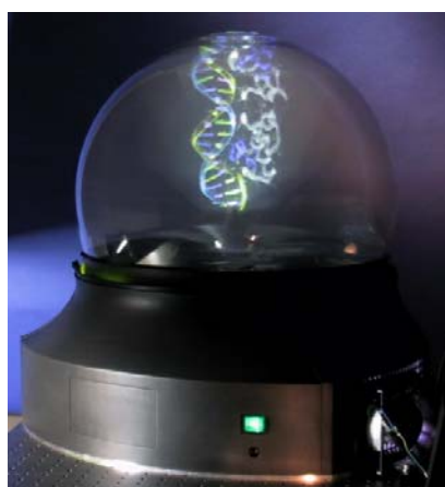
Pic 5: DNA molecule visualized by a volumetric display. (Image downloaded from Actuality System Inc. - http://www.actuality-systems.com/ )
