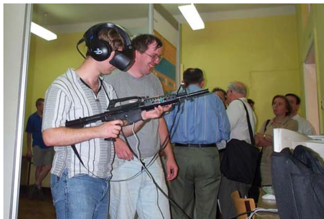
Pic 4: Using the HMD as an interface for MCE_VR electron maps visualization software. The gun serves for placing atoms in correct positions in the model.
