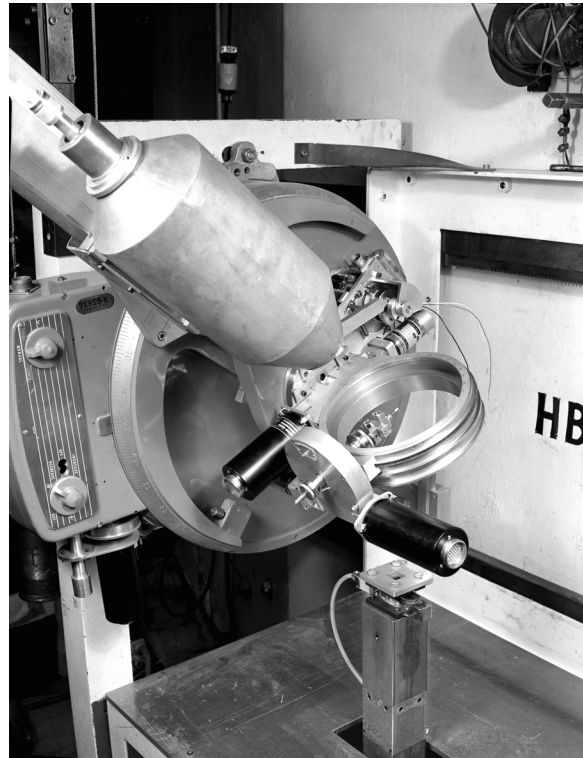
Fig. 2.: The three-circle paper-tape controlled neutron diffractometer at the Oak Ridge Research Reactor. (Photograph courtesy of ORNL)
