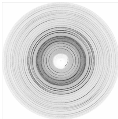
Fig. 9. Imaging plate frame for the orientation \psi = 30^\circ collected on the textured sample of AlPO-M. Note the differences in intensity around the rings.
