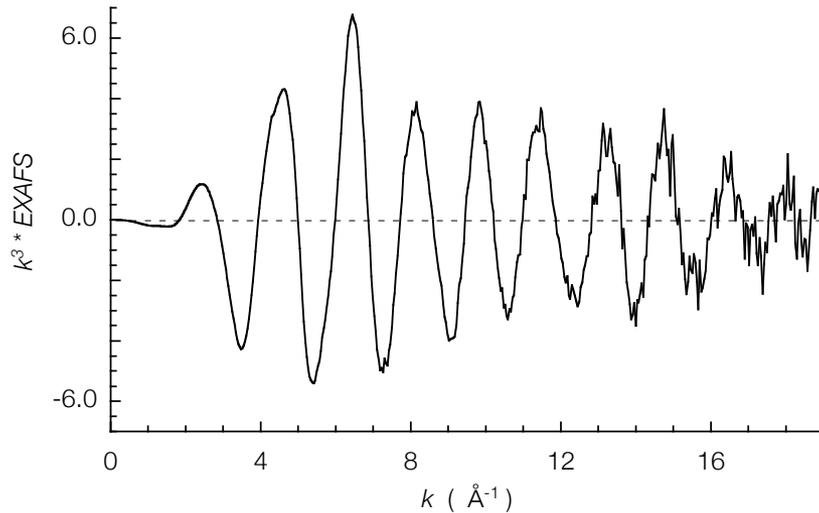
The final EXAFS is multiplied by  $k^3$  to compensate for the rapid attenuation with energy.
