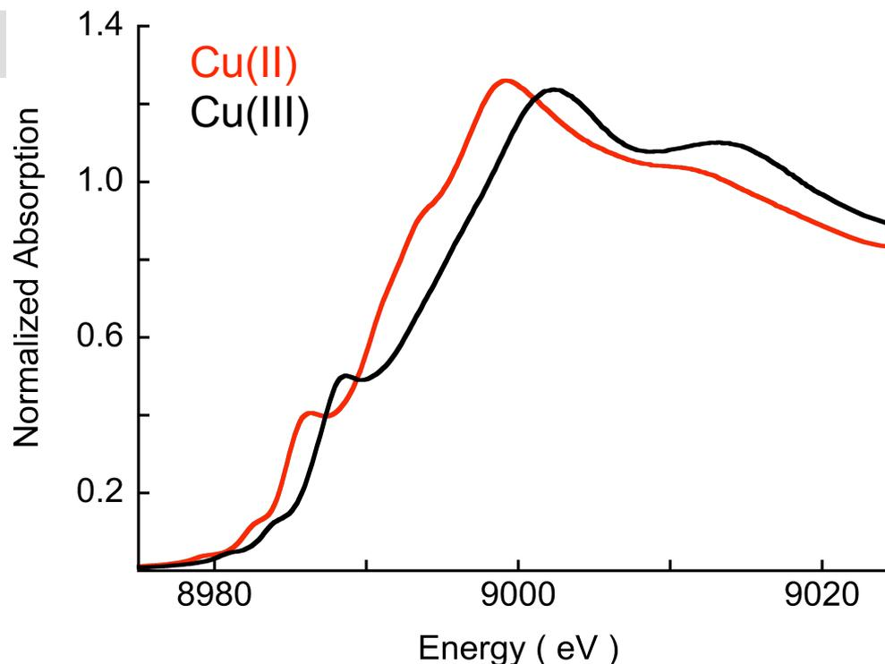
The rising-edge and the edge maxima shift to higher energy as the oxidation state increases.
