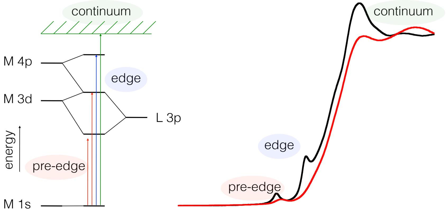
Metal K-pre-edge absorptions arise due to a quadrupole-allowed dipole-forbidden  $1s \rightarrow 3d$  excitation ( $\Delta l = \pm 2$ ) - weak
