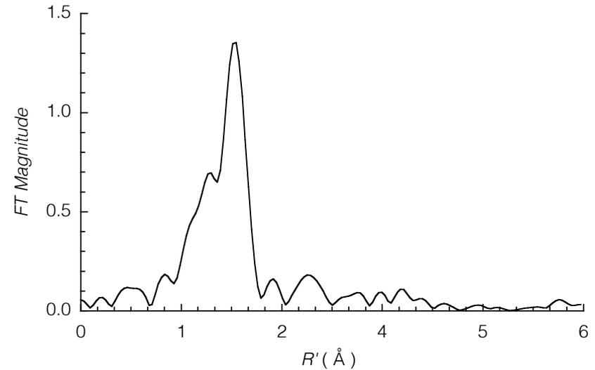
Fourier Transform (FT) is performed over a chosen  $k$  range to yield the radial distribution.
