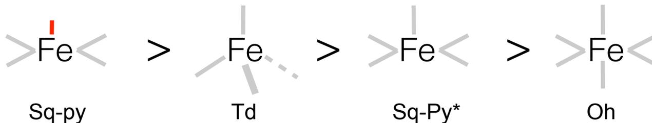
Pre-edge intensity  $\propto$  Deviation from Centrosymmetry  $\propto$  Metal 3d-4p mixing
