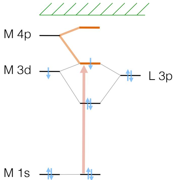
Pre-edge intensity  $\propto$  Deviation from Centrosymmetry  $\propto$  Metal 3d-4p mixing
