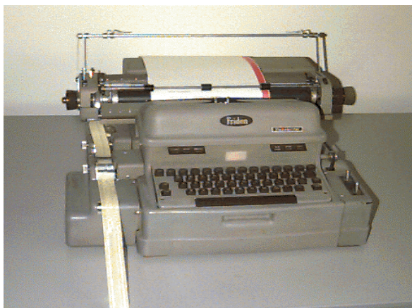
Flexowriter for the creation and editing of programs and data
