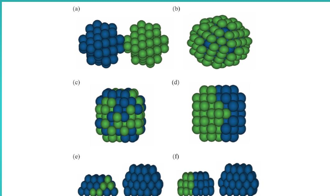
Fig. 9 Hypothetical bimetallic clusters (Pt = blue, Pd = green): (a) bi-cluster; (b) core-shell; (c) random; (d) single-half; (e) bi-cluster homo; (f) bi-cluster inhomogeneous.
