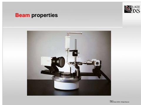
The properties of the X-ray beam depend on the X-ray tube (RAG/Sealed, type), optic (monochromator/multilayer optic), and collimator holes.
