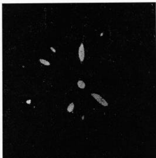
Fig. 12-6(2). Laue diffraction photograph of deformed single crystal of aluminium.
