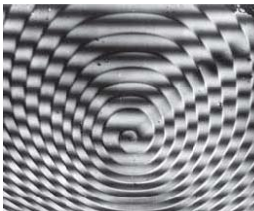
A spiral growth step on the silicon carbide surface.
