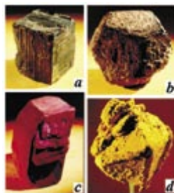
Natural (a, b) and synthesised (c, d) pseudomorphs, inheriting (a, c) and losing (b, d) the primary face relief. a, b – goethite after pyrite (Mining Museum collection, St. Petersburg), c – copper chromates after copper vitriol; d – potassium chromates after alum.
