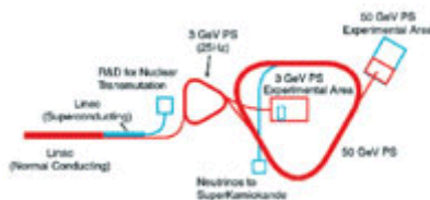
Fig. 3-3-1 A schematic layout of five major facilities based on an intense proton accelerator for the J-PARC jointly promoted by JAERI and KEK.
