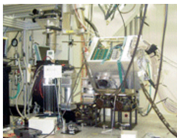
Fig. 2 The MSGC detector set up at SPring-8. The detector and the data acquisition system are installed in a cubic box of ca. 25 cm. Rotating the crystal around a vertical axis by 360 degrees on the goniometer, the intensity data can be observed within 0.2 msec.
