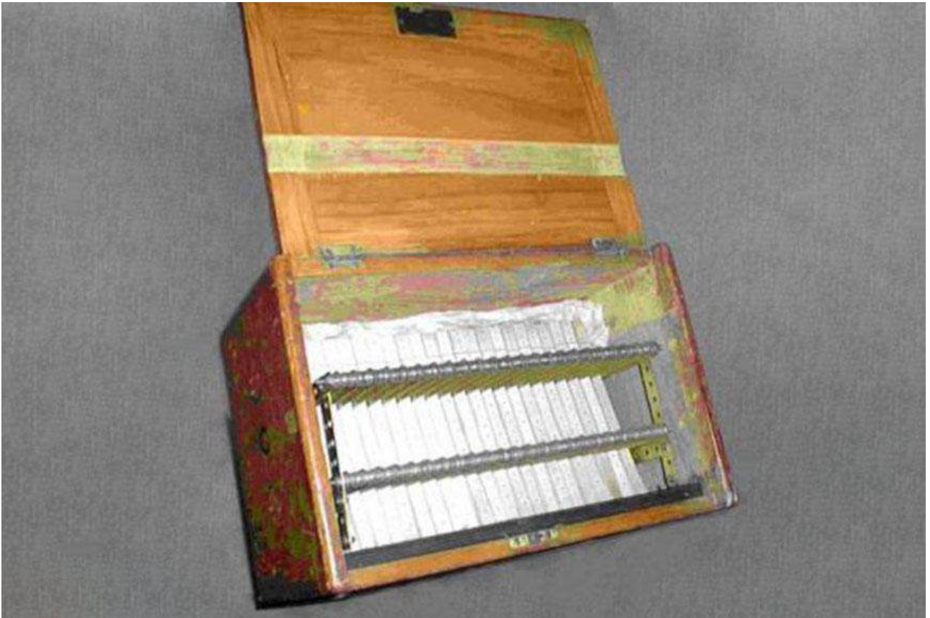
Figure 2. Prototype 6° cosine box of Beevers-Lipson strips. The boxes exported to other laboratories had sloping sides to ensure that when a strip was removed its place was left open for its re-insertion.
