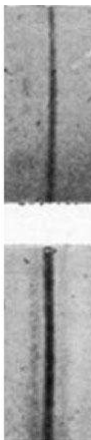
Figure 5 Extra side-band powder diffraction lines observed in a Cu, Fe, Ni alloy by Daniel & Lipson in 1942[xi].
