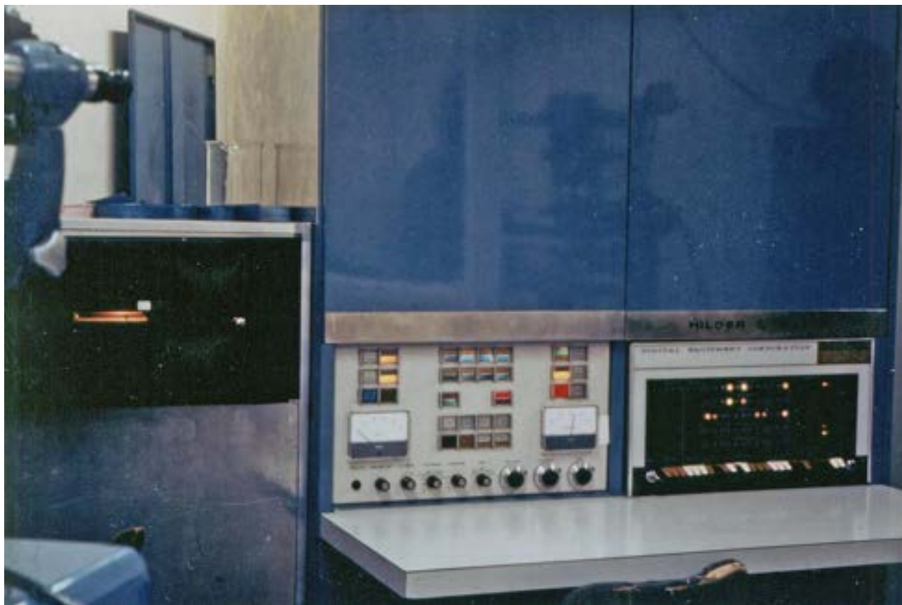
Figure 3. The control electronics for a Y290 diffractometer, including the PDP-8 minicomputer.
