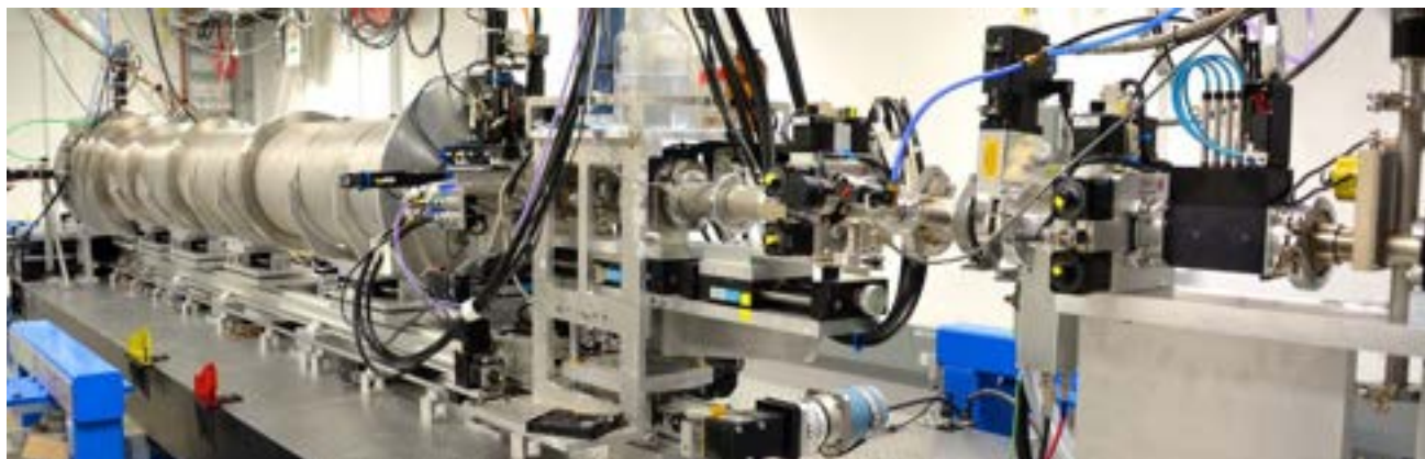
Figure 2. SAXS experimental station at SSRL used for COVID-19 research (Ivan Rajkovic, SSRL).
