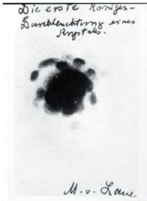
Figure 4. The first diffraction pattern of chalcantite, taken by Friedrich and Knipping and signed by Laue, in the shape of a Munich beer mug.
